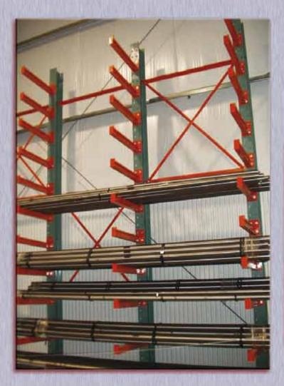
tion adjustable on 4" centers. The column to base connection is bolted using 6 to 12 bolts per side depending on the column/base size. One base is used for single-sided storage and two bases are provided for double-sided. Arm and column capacities vary depending on arm length and quantity and column height.
