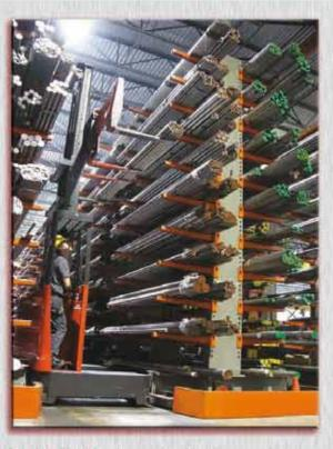
Guide Rails allow side loaders quick and easy access in narrow aisle applications. The Rail-to-Rail configuration maximizes storage space in narrow aisle applications. The Guide Rails are welded inside the rack's perimeter saving valuable floor space.
