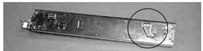
Figure 15 Slide Detail Showing Large hook
